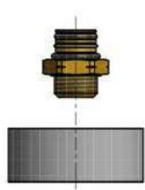
The fit the component by means of push and twist.
