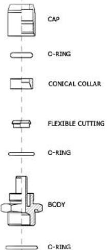
The **SIRIT** fittings for braking systems comply with **DIN 2353** regulation. The types of fittings shown in this catalogue are based on the requests made by the main European braking systems installers.
