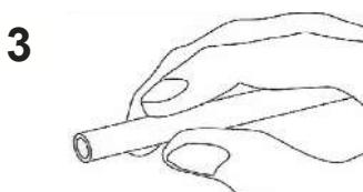
Prepare the tubing ready For insertion ensuring that the end is cut square
