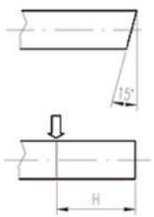
The tubing must be cut at the right angles with a maximum tolerance of 15°. Correct assembly is performed only when the tubing is inserted touches the end of the tube seat. To be absolutely certain that this is the case it is advisable to mark the depth of the tubing coupling (distance H).
