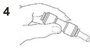
Insert tube, ensuring you have reached the stop position, now pull back
