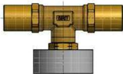
Screw the swivel Coupling into the thread ensuring the correct torque (Over-tightening can cause damage to both the fitting
