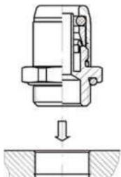
The seal of the stud coupling is specified by what is laid down in ISO standard 6149-80 and DIN standard 3482. To obtain the correct assembly on all terminal fittings it is essential to adhere to the tightening torques shown in the following table:
