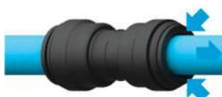
**TO DISCONNECT, ENSURE THE SYSTEM IS DE-PRESSURISED. PUSH THE COLLET TOWARDS THE FITTING AND REMOVE THE PIPE**
