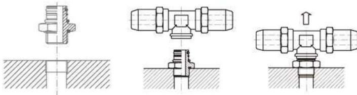
Screw the swivel coupling into the thread ensuring correct torque
